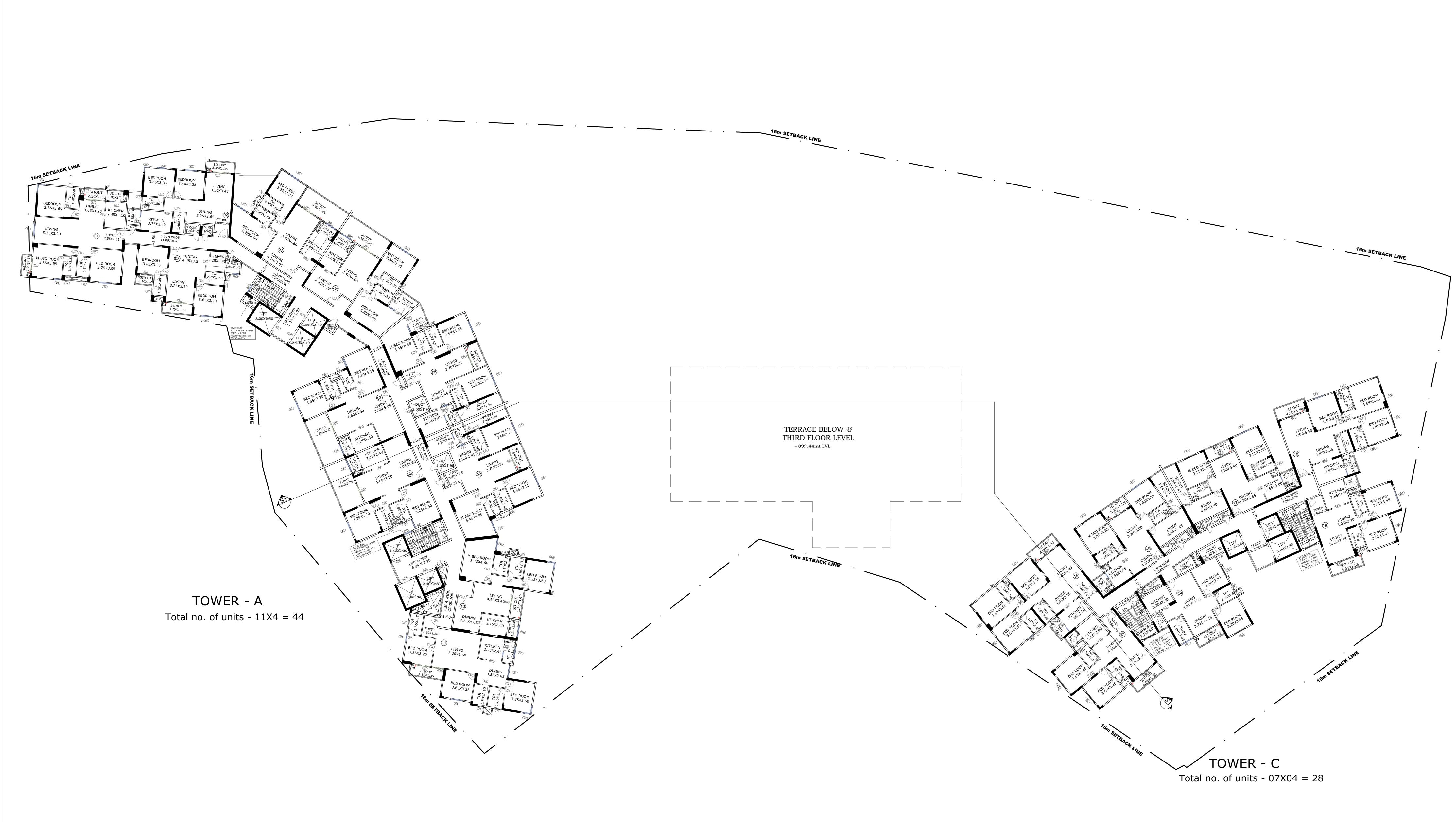
TYPICAL 5th, 9th, 17th, 21st FLOOR PLAN +898.44mt LVL, +910.44mt LVL, +934.44mt LVL, +946.44mt LVL Total no. of units - 07X04 = 28
